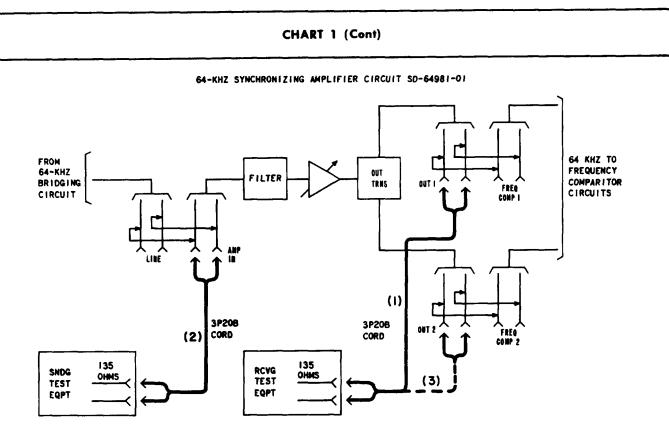
Fig. 2—64-kHz Synchronizing Frequency Amplifier—Gain Measurement
