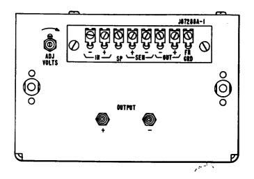
Fig. 1—DC-to-DC Converter (Front View)
