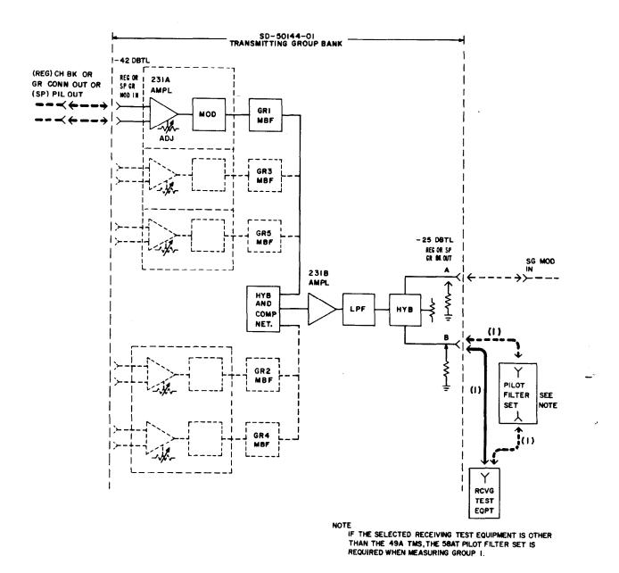
Fig. 1—Group Modulator In-Service Gain Test
