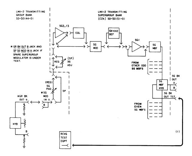
Fig. 4—Supergroup Modulator In-Service Loss Test
