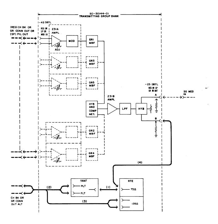
Fig. 8— N3-L Group Modulator In-Service Gain Test
