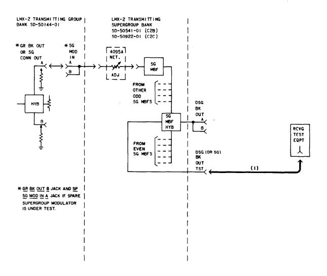
Fig. 7—Supergroup Modulator In-Service Loss Test
