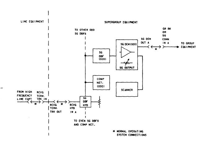
Fig. 3—Receiving Supergroup In-Service Connections—Simplified Block Diagram
