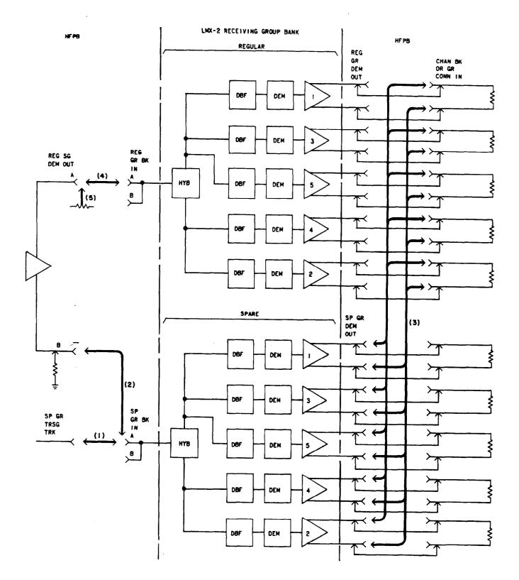
Fig. 2-Removing Regular Receiving Group Bank from Service
