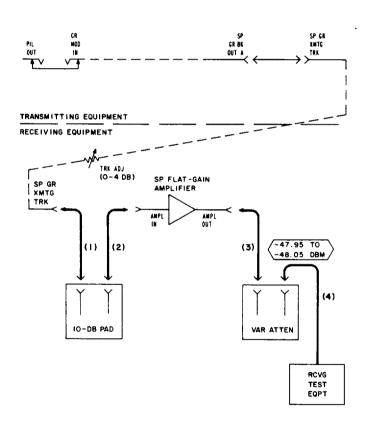
Fig. 1—Pilot Level Test Connections
