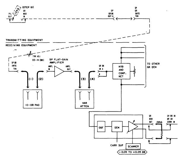
Fig. 2—\$Test Connections for Amplifier Adjustments
