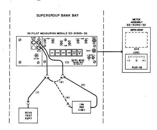
Fig. 1—315.92 kHz Pilot Measuring Circuit Calibration For J68918 Scanner
