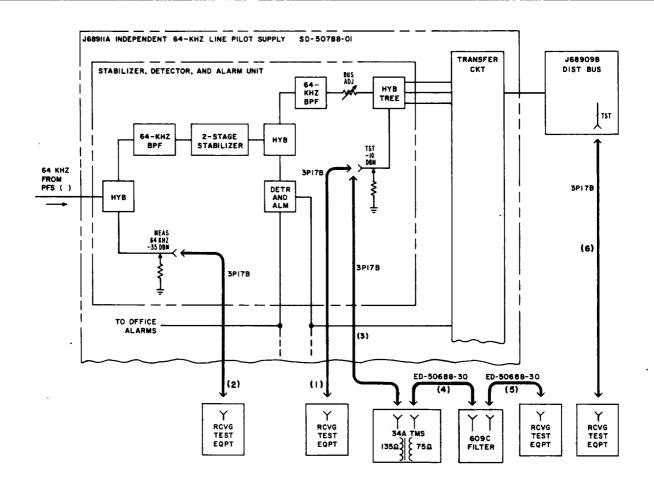
Fig. 4—Mndependent 64-kHz Pilot Supply and Distribution Bus Test Connections
