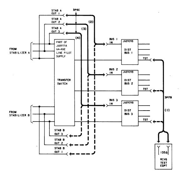
Fig. 5—\$Transfer Switch Replacement or Failure—Patching Procedures\$
