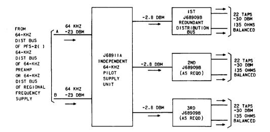
Fig. 2-Independent 64-kHz Supply and Distribution Circuit
