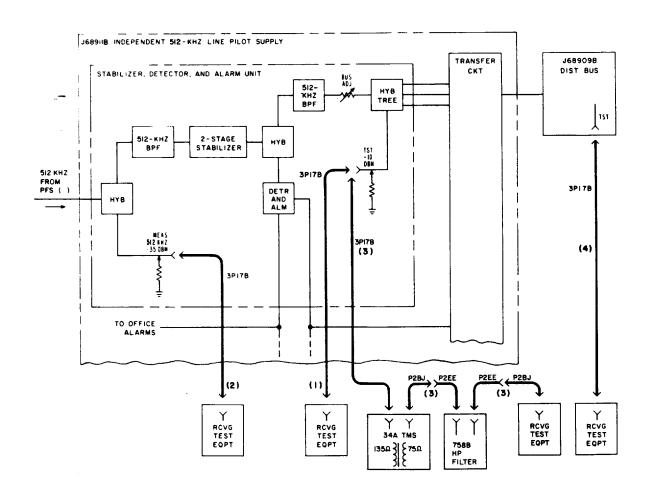
Fig. 3—Independent 512-kHz Pilot Supply and Distribution Circuit Test Connections
