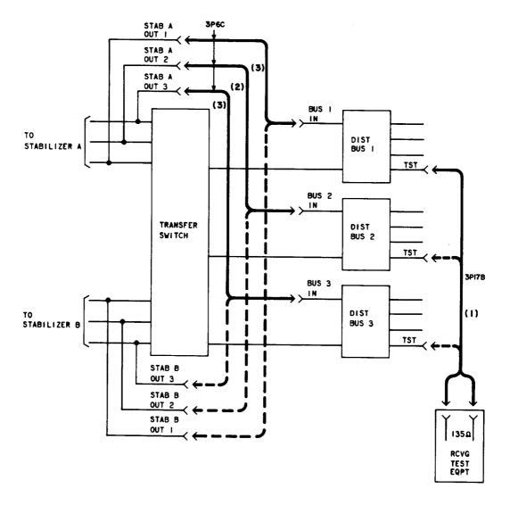
Fig. 4—Transfer Switch Replacement or Failure—Patching Procedures
