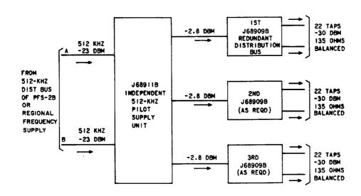
Fig. 2—Independent 512-kHz Pilot Supply and Distribution Circuit
