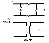
Fig. 5 — ON/K-to-ON Connecting Circuit Input
