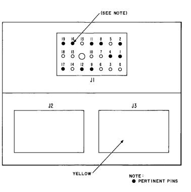
Fig. 3 — Repeater Mounting Bracket with Repeater Removed
