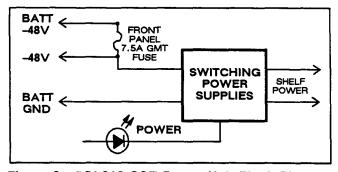
Figure 2. DDL210 COT Power Unit Block Diagram
