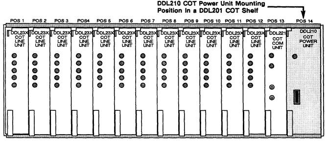
Figure 3. Typical DDL210 COT Power Unit Mounting Position (Front View)
