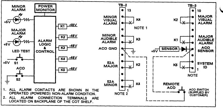
Figure 2. DDL221 COT Common Unit Block Diagram
