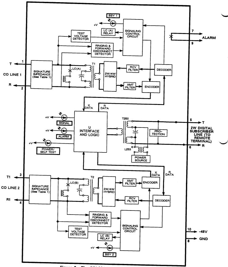
Figure 3. The DDL391 Line Unit Block Diagram
