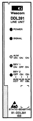
Figure 1. DDL391 Line Unit
