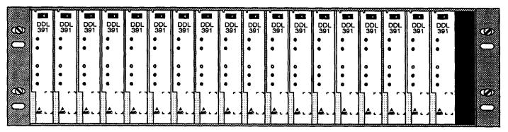
Figure 4. Shelf Showing DDL391 Line Unit Mounting
