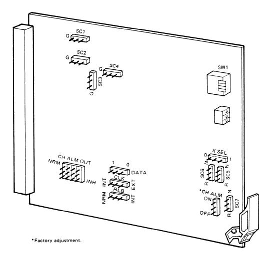
Figure 5-10 MUX Unit (Grp: 0A00/0B00) Straps Location (Sheet 1 of 2) #
