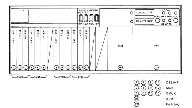
(H) Bipolar Interface of Non-redundant Configuration for AC Application
