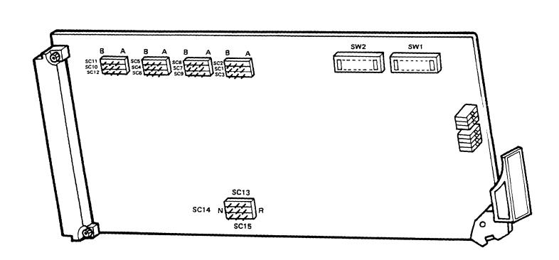
Fig. 5-7A DMUX Unit (GRP: 0A02/0B02) Options Location 4
