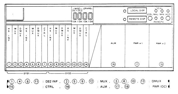
(C) Bipolar Interface of Redundant Configuration for DC Application
