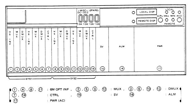
(E) Optical Interface of Redundant Configuration for AC Application
