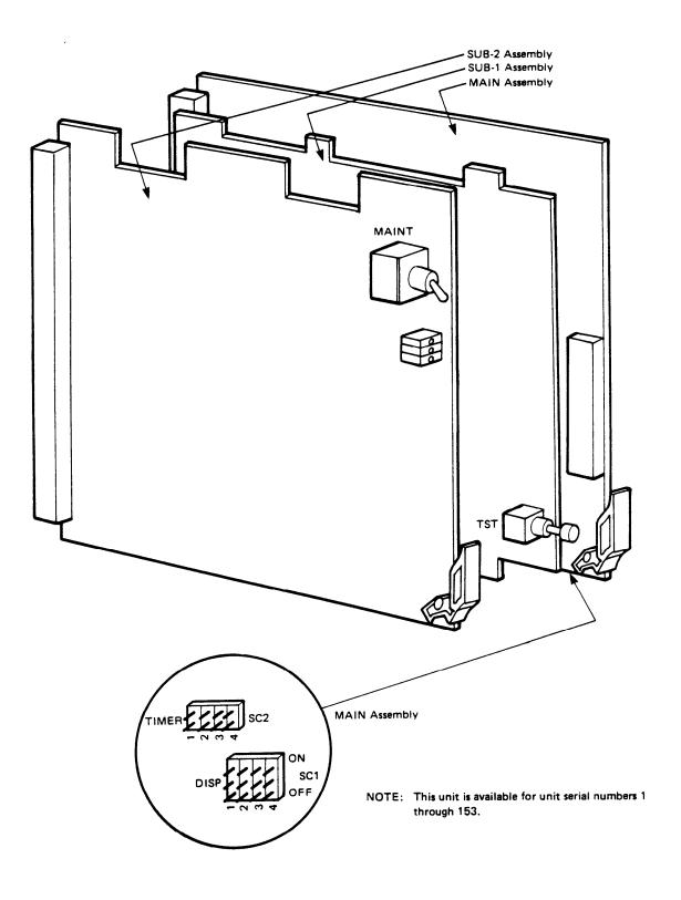
Figure 5-1 ALM Unit (Grp: 0A00) Straps Location (Sheet 1 of 2)
