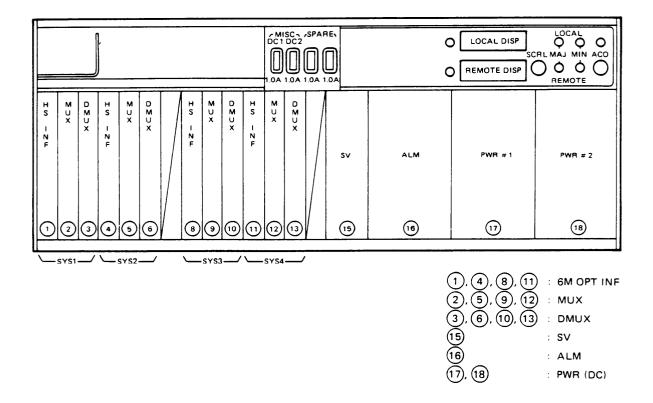
(B) Optical Interface of Non-redundant Configuration for DC Application
