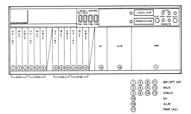
(F) Optical Interface of Non-redundant Configuration for AC Application
