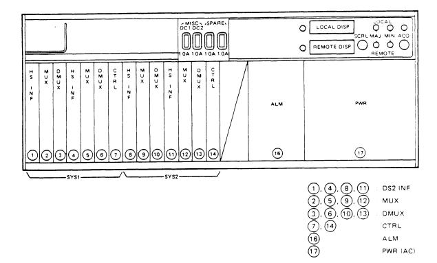
(G) Bipolar Interface of Redundant Configuration for AC Application
