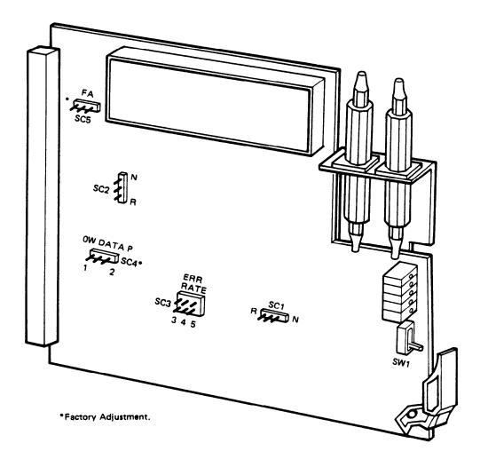
Figure 5-11 6M OPT INF (X0306) Unit (Grp: 0E00, 0F00, 0F01) Straps Location (Sheet 1 of 2)
