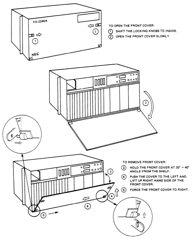
Figure 3-2 Front Cover Removing Method
