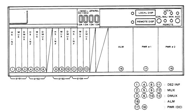
(D) Bipolar Interface of Non-redundant Configuration for DC Application
