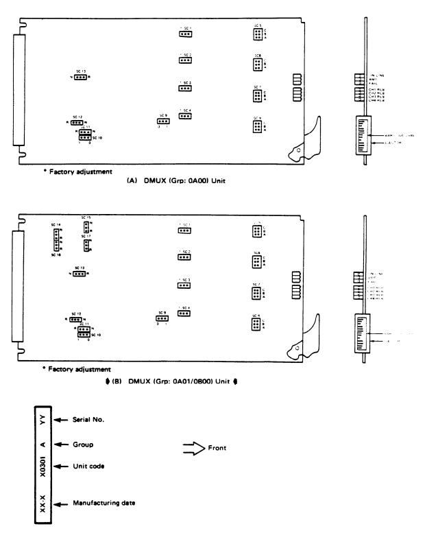
NOTE: Printed on the right side surface of the main board connector.
