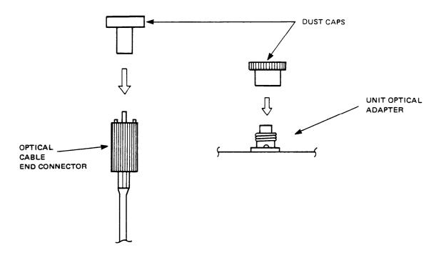
Figure 4-1 Installing Protective Dust Caps
