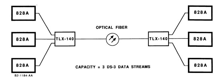
Figure 1-7. 828A Digital Multiplexer in a TLX-140 Fiber-Optic Transmission System
