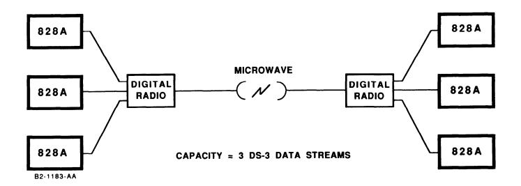
Figure 1-6. 828A Digital Multiplexer in a Digital Microwave System
