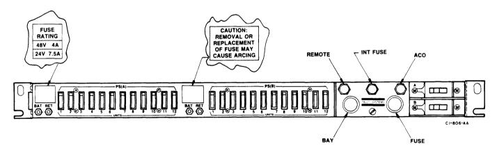
Figure 1-3. ACX025 Fuse and Alarm Panel
