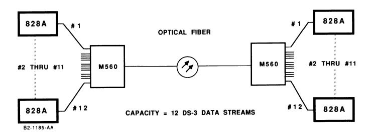
Figure 1-8. 828A Digital Multiplexer in an M560 Fiber-Optic Transmission System
