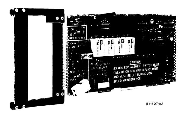
Figure 1-5. Maintenance Interface Card
