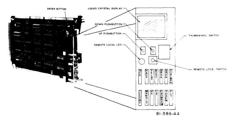
Figure 2-7. Manual Control Interface Card
