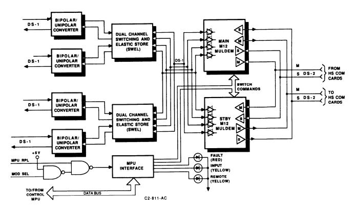
Figure 2A-3. LS INTER T1 Card Block Diagram
