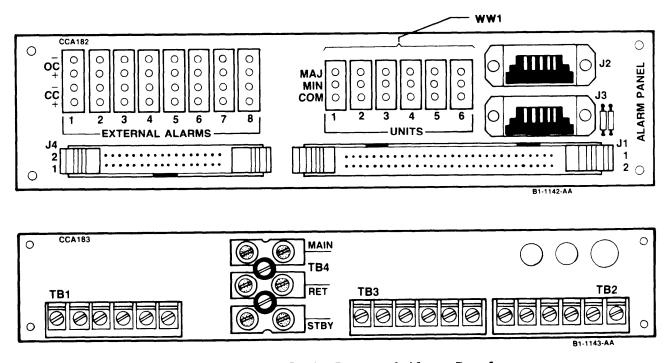
Figure 2-4. ACXO43 Fuse and Alarm Panel
