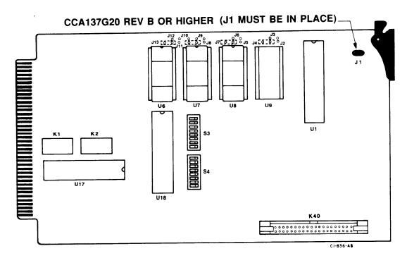
Figure 2F-1. Control MPU Card (CCAl37)
