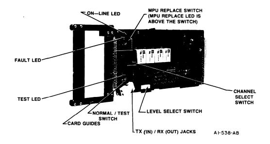
Figure 2-5. Maintenance Interface Card
