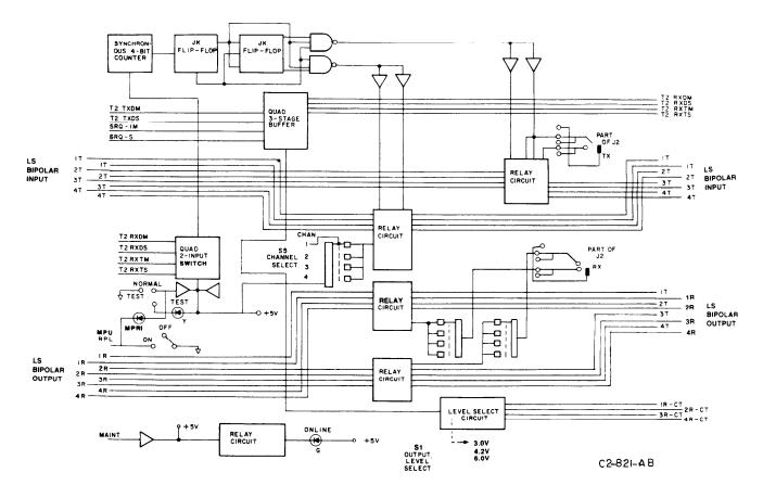
Figure 2-6. Maintenance Interface Card Block Diagram
