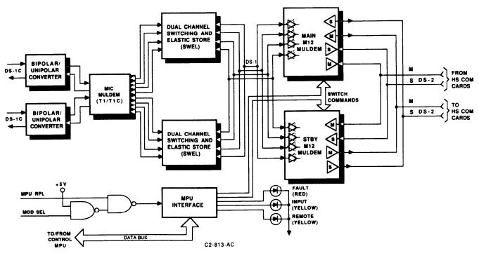
Figure 2A-4. LS INTER T1C Card Block Diagram
