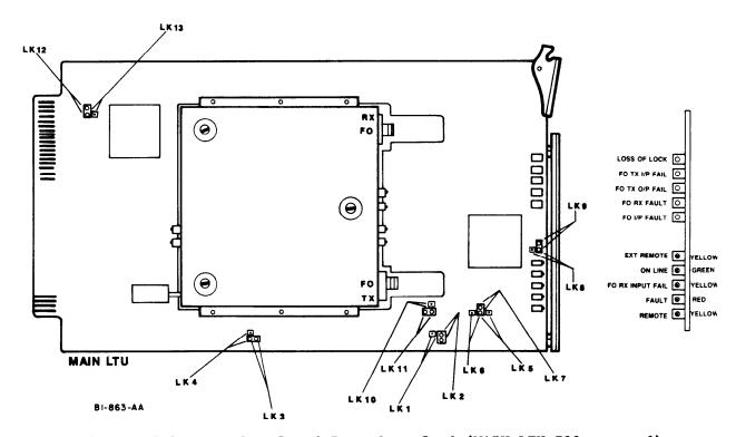
Figure 2C-1. LTU Low-Speed Interface Card (MAIN LTU Illustrated)
