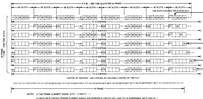
(2) M0 M1 M0 IS THE MULTIFRAME ALIGMENT SIGNAL AND APPEARS IN THE 5TH, 6TH, AND 7TH M SUBFRAMES. MO-O AND M1-1
