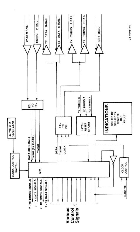
Figure 2D-1. HS COM Card Block Diagram
