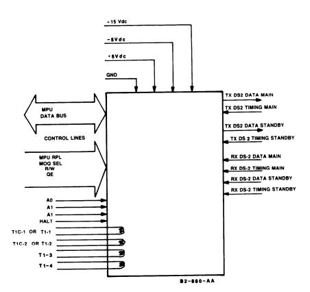
Figure 2A-2. LS INTER T1/T1C Card Interfaces
