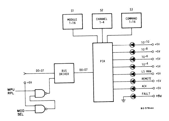
Figure 2-8. Manual Control Interface Card Block Diagram
