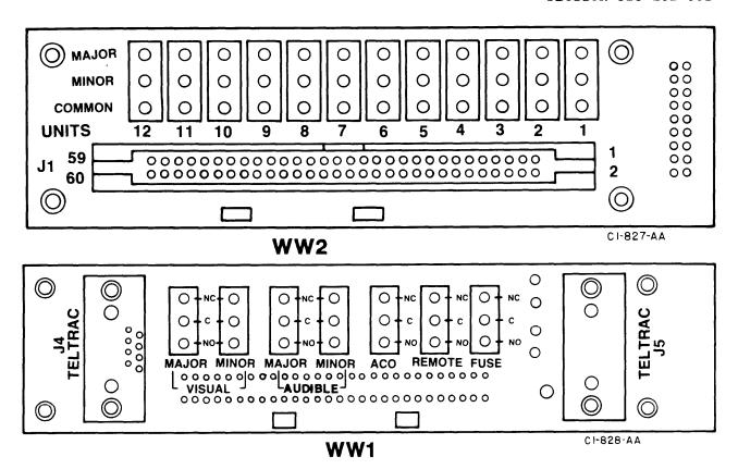
Figure 2-3. ACX025 Fuse and Alarm Panel
