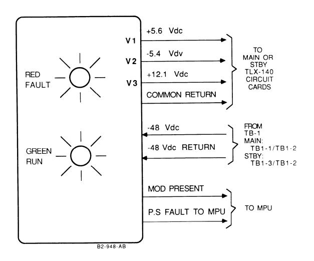
Figure 2H-2. PS Module Interfaces
