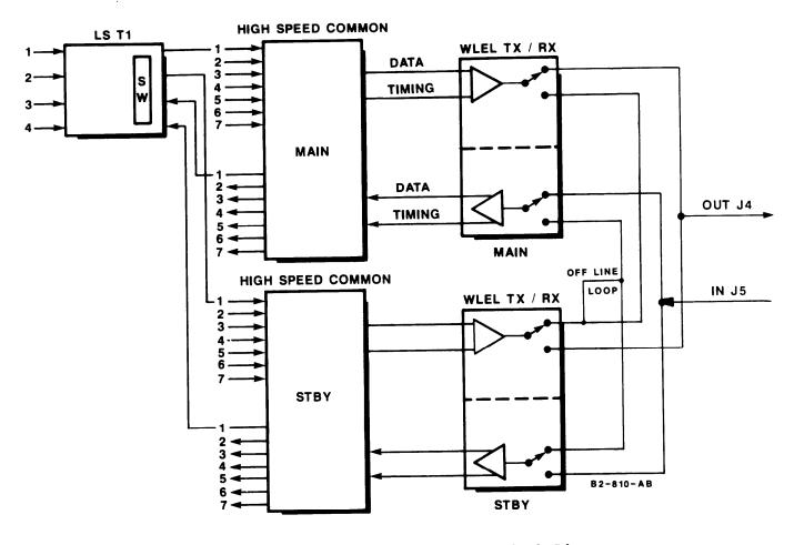
Figure 2-2. 828A Digital Multiplexer Block Diagram
