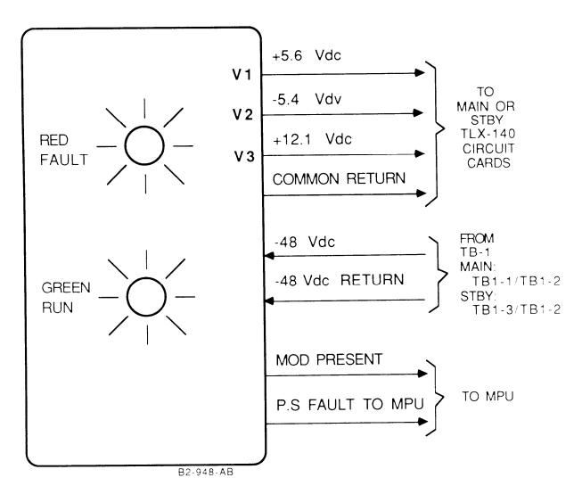
Figure 2H-2. PS Module Interfaces
