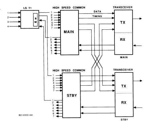
Figure 2-2. 828AF Digital Multiplexer Block Diagram
