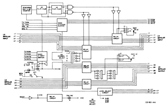
Figure 2-6. Maintenance Interface Card Block Diagram
