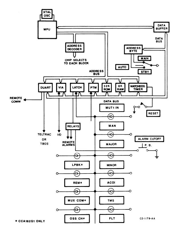
Figure 2F-3. Control MPU Card Block Diagram
