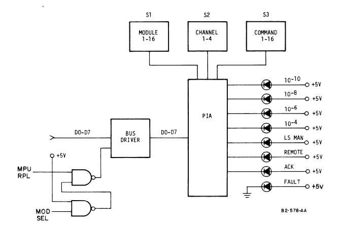
Figure 2-8. Manual Control Interface Card Block Diagram
