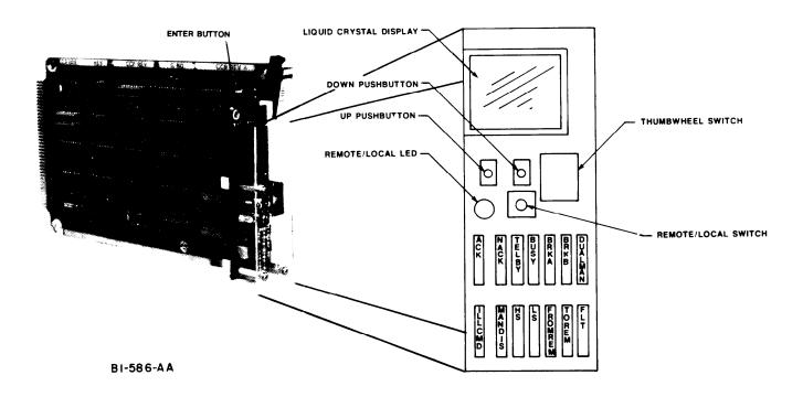
Figure 2-7. Manual Control Interface Card
