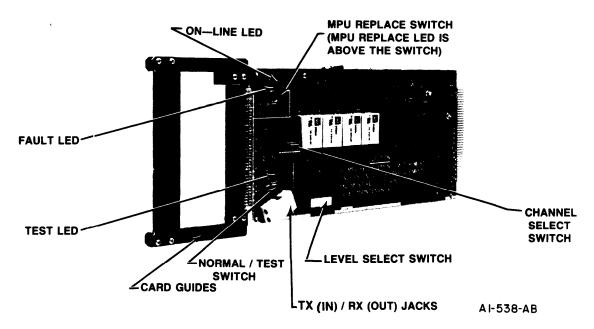
Figure 2-5. Maintenance Interface Card
