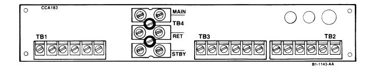
Figure 2-4. ACX043 Fuse and Alarm Panel
