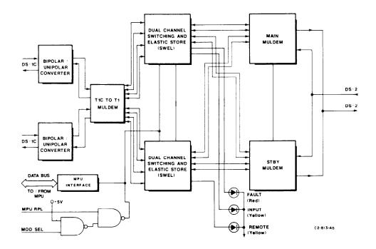
Figure 2A-4. LS INTER TIC Card Block Diagram
