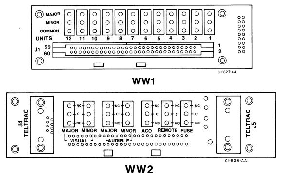
Figure 2-3. ACX025 Fuse and Alarm Panel
