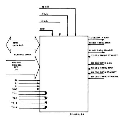
Figure 2A-2. LS INTER T1/T1C Card Interfaces
