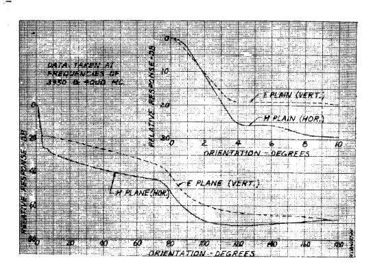
Fig. 3 – Maximum Response Curves for KS-5759 Antenna
