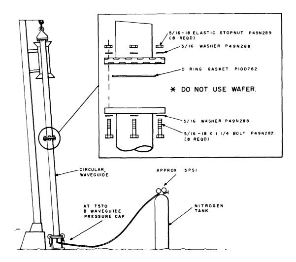
Fig. 7—Joining Circular Waveguide Sections—One Flange With Integral Gasket Groove
