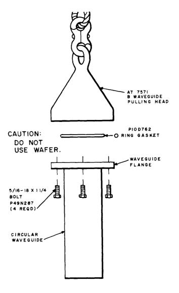
Fig. 3-Attachment of Pulling Head
