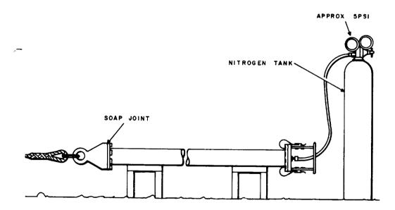
Fig. 5—Pressure Test of Pulling Head Connection
