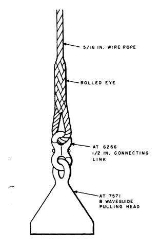
Fig. 2—Attachment of Winch Line to Pulling Head
