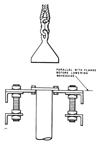
Fig. 12-Securing Circular Waveguide
