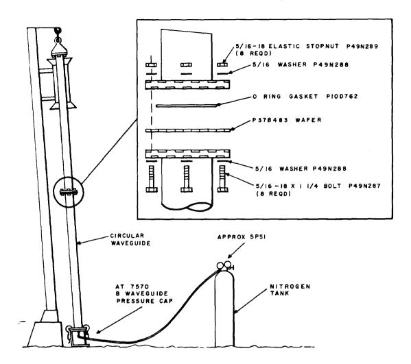
Fig. 9-Joining Circular Waveguide Sections—Forged Flanges
