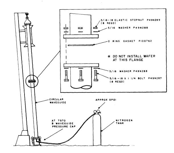
Fig. 8—Joining Circular Waveguide Sections—Both Flanges With Integral Gasket Grooves
