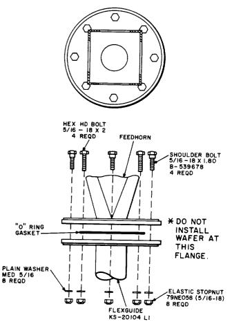
Fig. 13—Installation of Flexible Waveguide at Feedhorn
