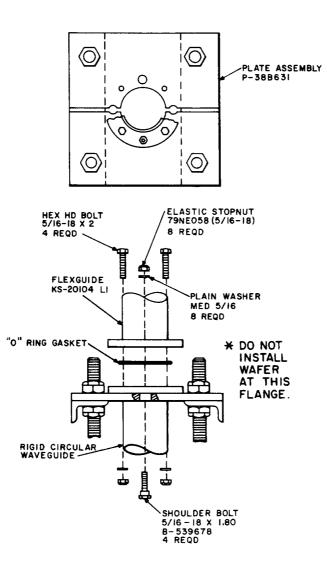
Fig. 14—Installation of Flexible Waveguide at Hanger Plate
