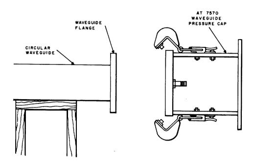
Fig. 4—Attachment of Pressure Cap
