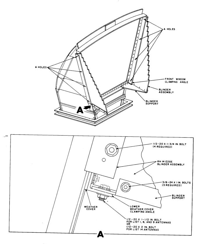
Fig. 14—Side View of KS-15676 Antenna With the Blinder Assembly
