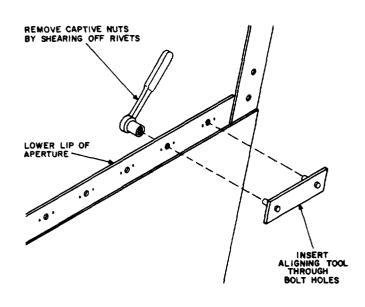
Fig. 9—Removing Captive Nuts
