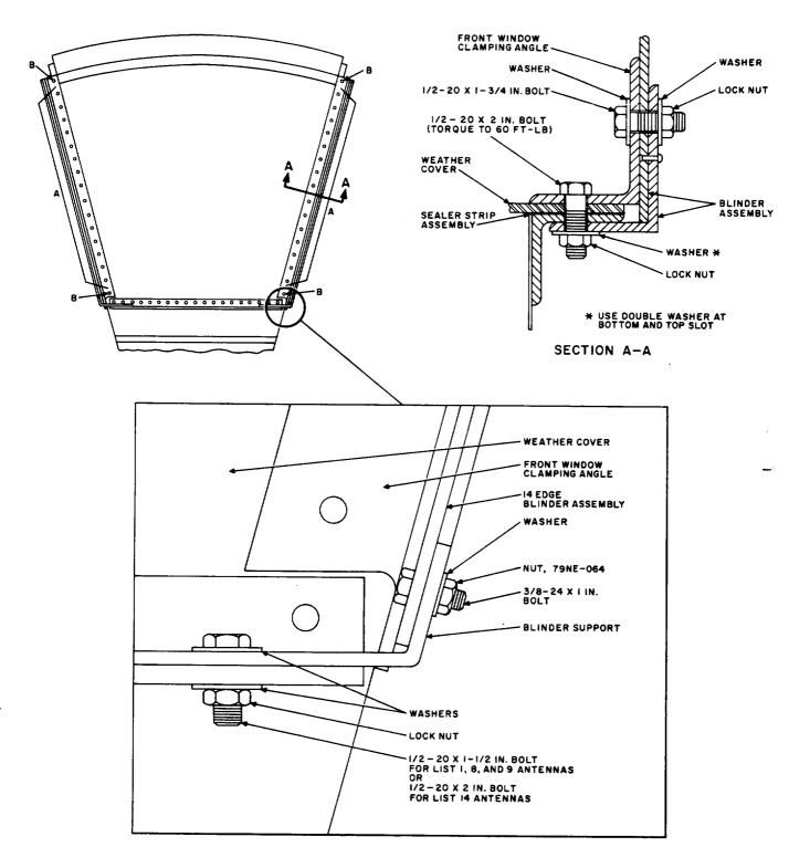
Fig. 13—KS-15676 Antenna Face and Blinder Assembly
