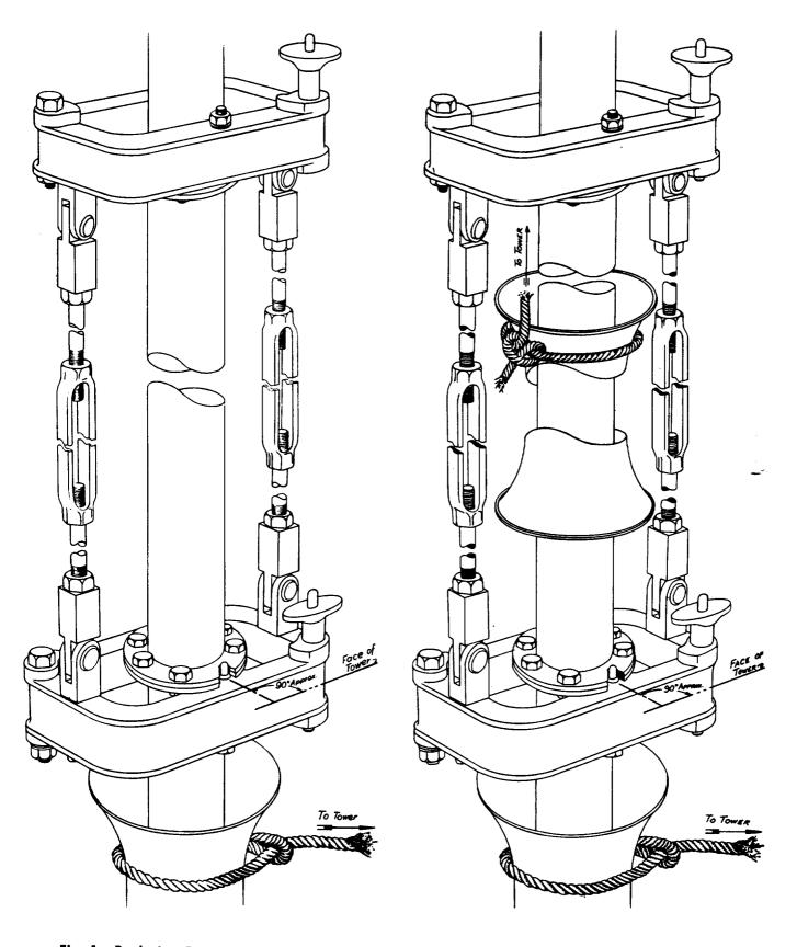
Fig. 1 – Replacing Damaged Waveguide
