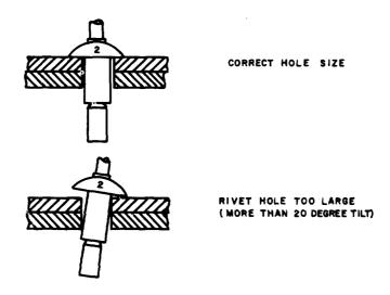
Fig. 1—Rivet Placement
