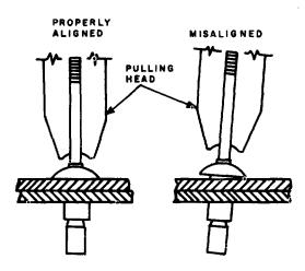
Fig. 2—Pulling Head Placement
