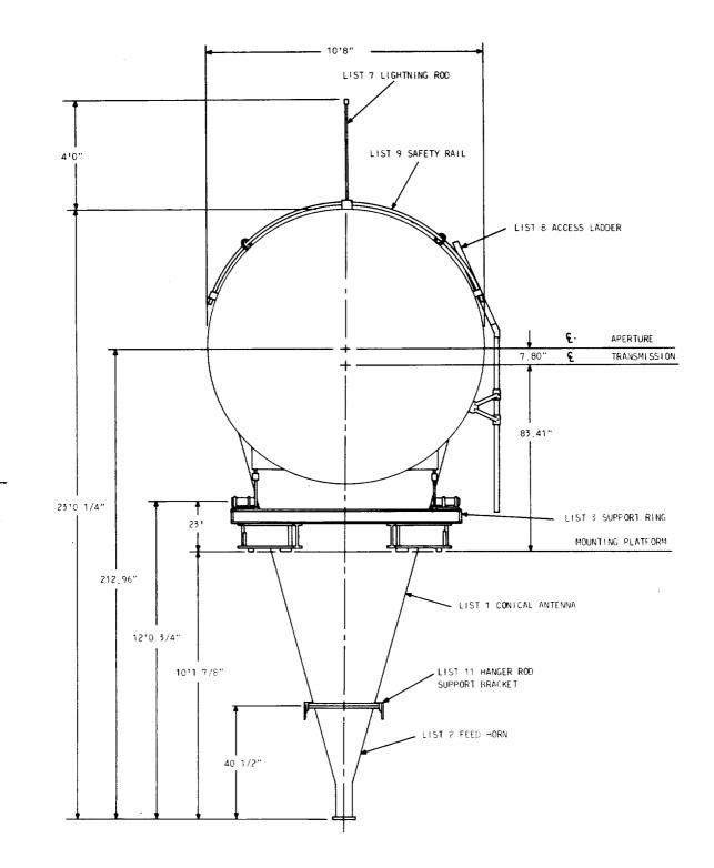
Fig. 1—KS-21972 Conical Antenna (Front View)
