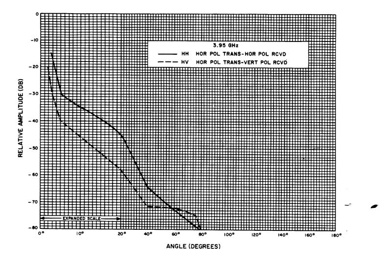
Fig. 4—KS-21972 Conical Antenna, 3.95 GHz, Horizontal Polarization Transmitted
