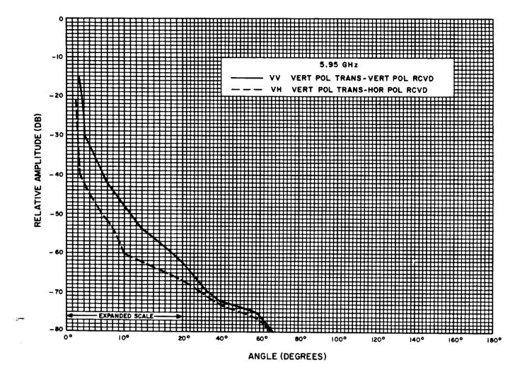
Fig. 5—KS-21972 Conical Antenna, 5.95 GHz, Vertical Polarization Transmitted
