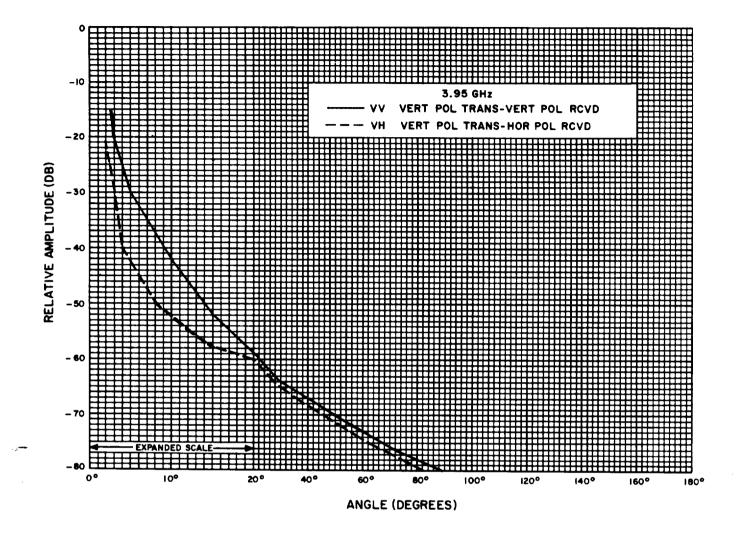
Fig. 3—KS-21972 Conical Antenna, 3.95 GHz, Vertical Polarization Transmitted
