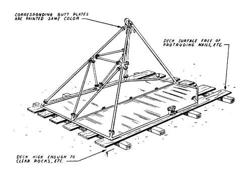
Fig. 2 — Method of Assembling KS-16320 Passive Reflector
