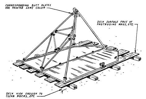
Fig. 2 — Method of Assembling KS-16320 Passive Reflector
