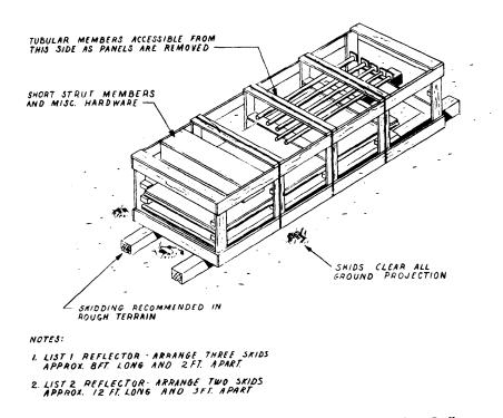
Fig. 1 — Placement of Shipping Crate for KS-16320 Passive Reflector
