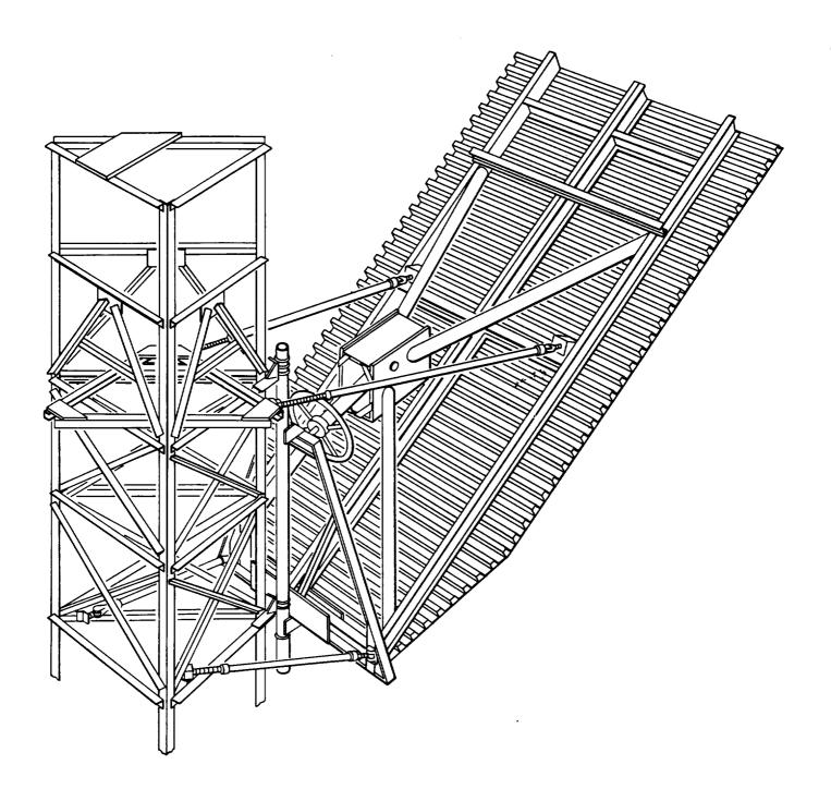
Fig. 1—KS-19570 L3 Passive Reflector—Typical Installation
