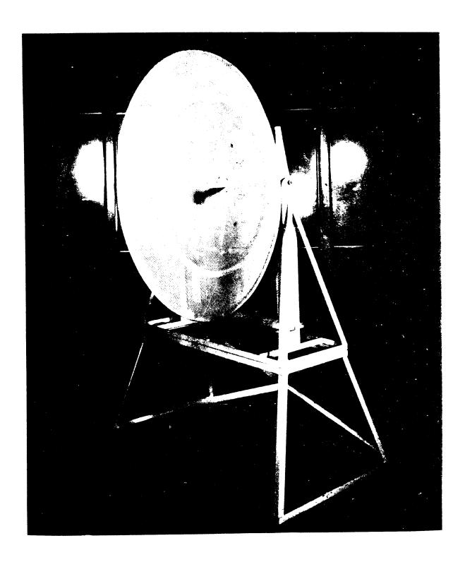
Photo A – Parabolic Reflector Antenna Assembly Reflector Diameter-57" (Wave Guide Feed Oriented for Vertical Polarization)
