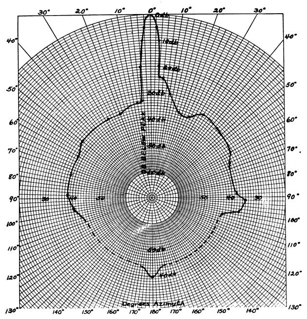
Note: This curve indicates the values of the envelope of the radiation pattern measured at a given location. The dotted portion indicates levels less than 45 db which could not be measured.
