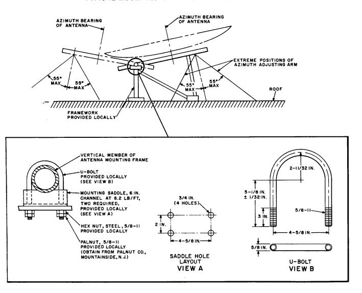
Fig. 18—Antenna Installation on Roof
