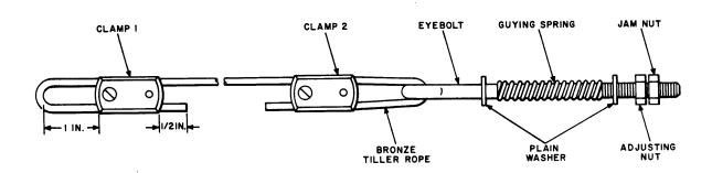
Fig. 9—Antenna Feed Guying Assembly
