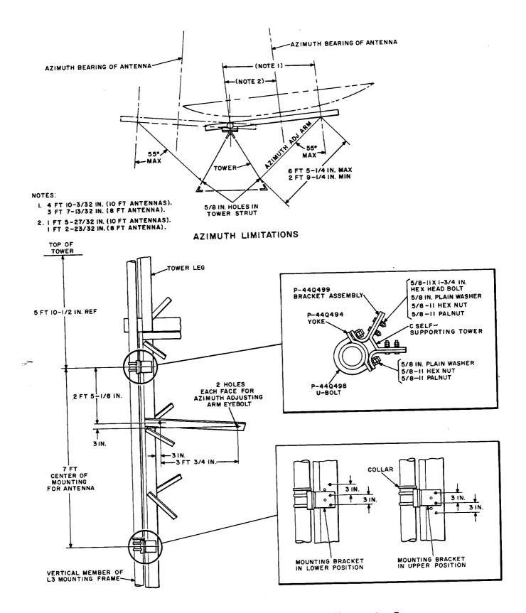
Fig. 17—Antenna Installation on AT-8013 C Self-Supporting Tower
