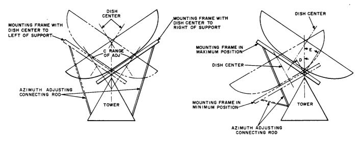
ARRANGEMENT OF ANTENNA AND MOUNTING FRAME TO OBTAIN MAXIMUM ADJUSTMENT
