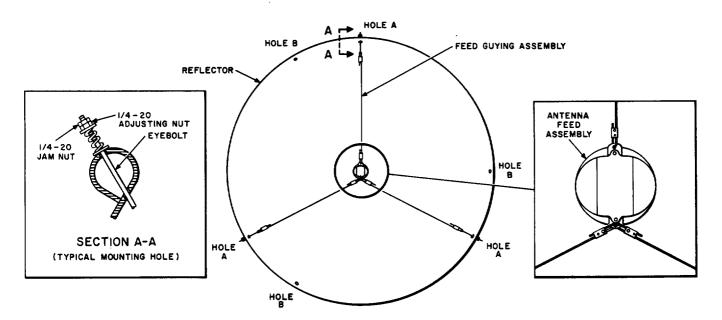
Fig. 10-Mounting Hole Configuration in Reflector Rim
