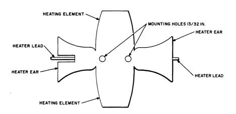
Fig. 12—Feed Heater Element (Technical Appliance Corporation)
