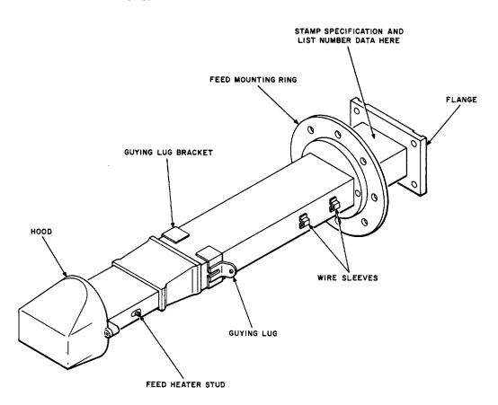
Fig. 6—Broadband Antenna Feed Assembly (Gabriel Electronics)
