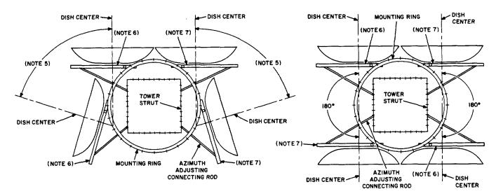
AZIMUTH LIMITATION OF ADJACENT ANTENNA WHEN TWO ANTENNAS ON THE SAME BEARING ARE MOUNTED ON THE SAME SIDE OF TOWER
