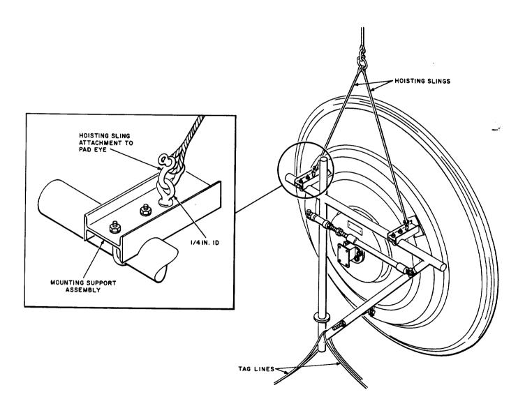
Fig. 14—Hoisting Sling and Tag-Line Attachments to Antenna
