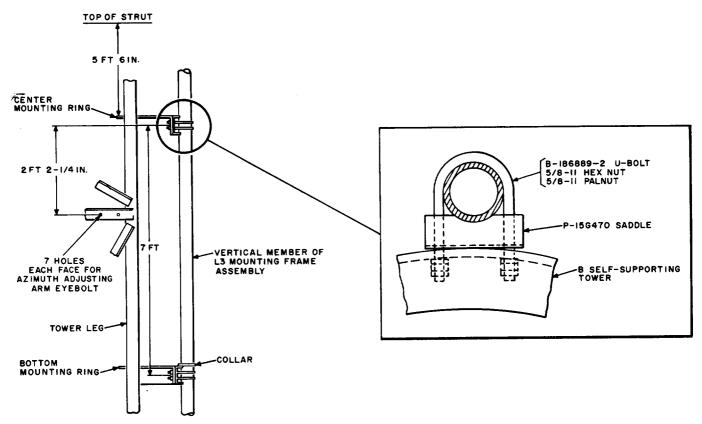
Fig. 16—Antenna Installation on AT-7729 B Self-Supporting Tower
