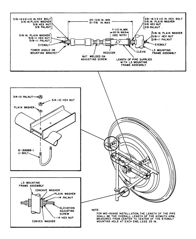
Fig. 5—Elevation Adjusting Screw and Azimuth Adjusting Arm
