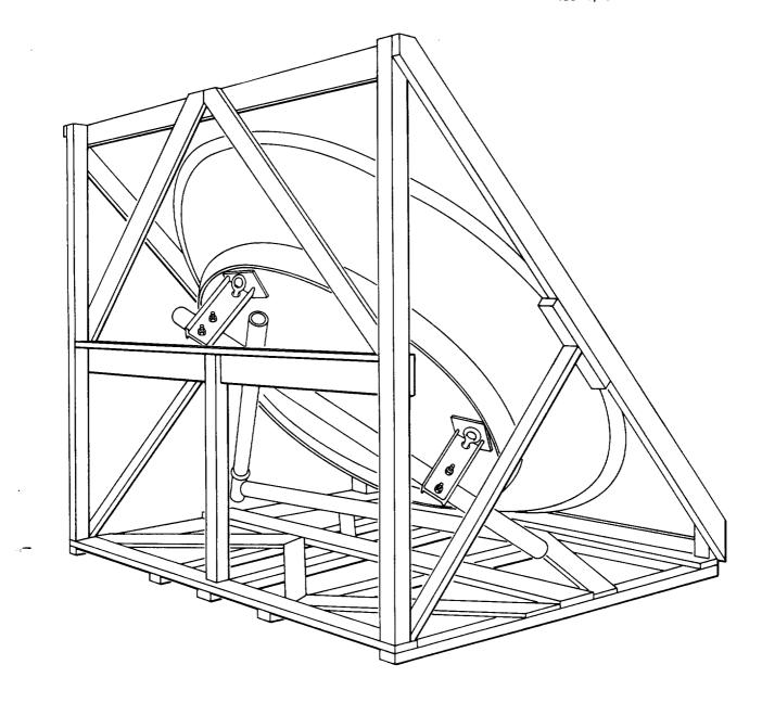
Fig. 2—Antenna in Shipping Crate
