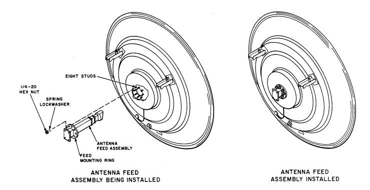
Fig. 8—Installation of Antenna Feed Assembly
