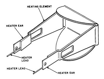
Fig. 11—Feed Heater Assembly (Gabriel Electronics)
