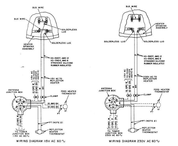
Fig. 13—Feed Heater and Reflector Heater Wiring Diagrams
