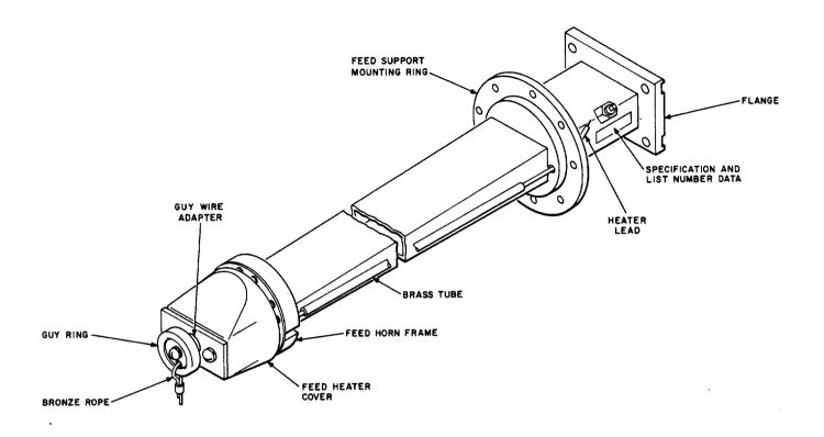
Fig. 7—Broadband Antenna Feed Assembly (Technical Appliance Corporation)
