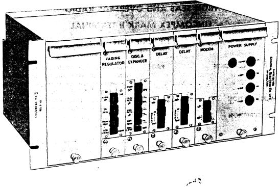
Fig. 2—Lincompex Receive Terminal
