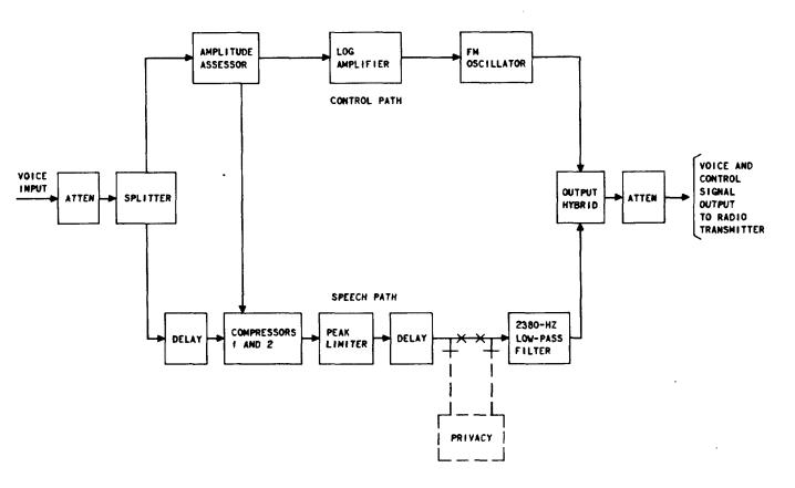
Fig. 8—Transmit Terminal—Block Diagram
