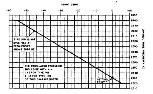
Fig. 4---Transmit: Input/Control Tone Frequency Characteristic
