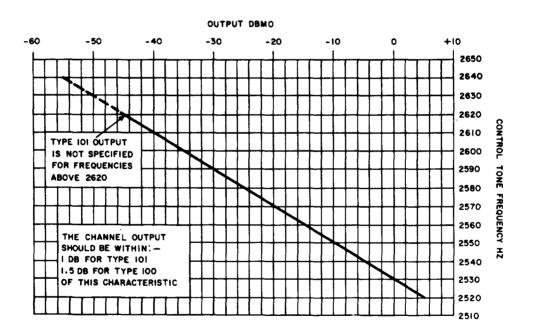
Fig. 6-Receive: Control Tone Frequency/Output Characteristic
