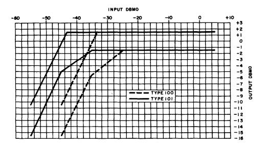
Fig. 3—Transmit: Compression Characteristic, Input/Output
