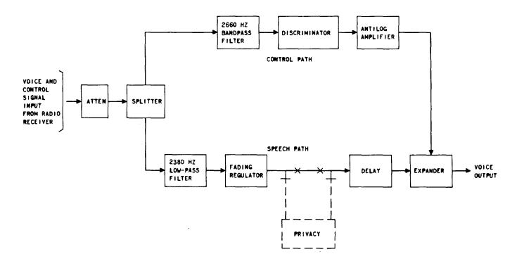
Fig. 9—Receive Terminal—Block Diagram
