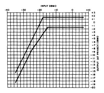
Fig. 5--Receive: Fading Regulator Characteristic Input/Output
