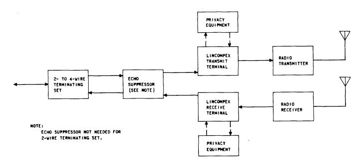
Fig. 2—Radiotelephone Terminal Arrangement
