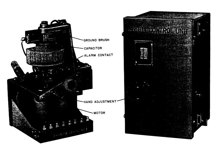
Fig. 1—50-A Automatic Frequency Control Unit
