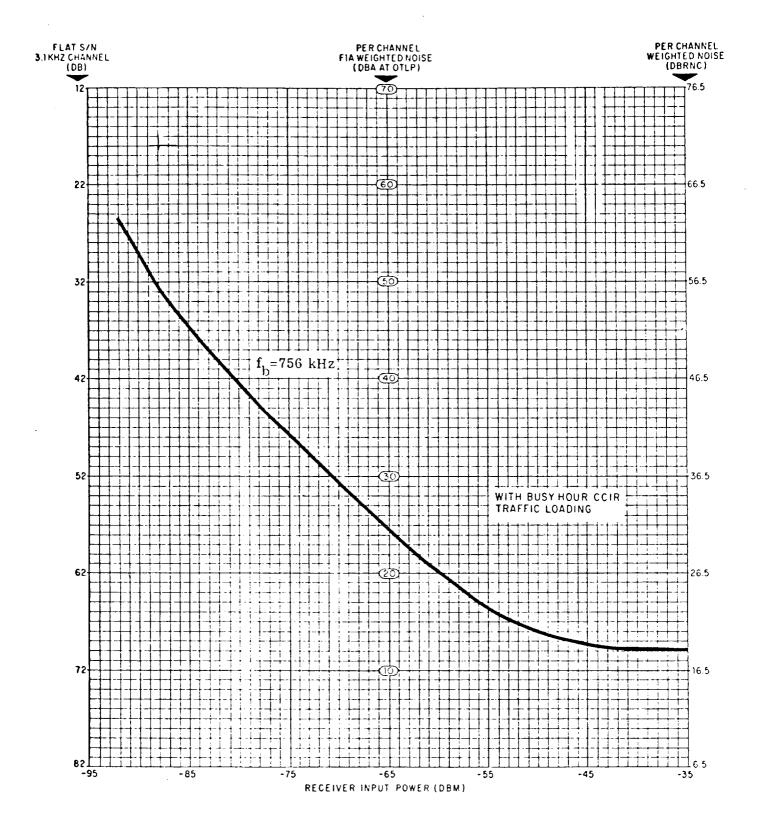
Fig. 6—Typical Performance Characteristics for SS2000W-02-70211 Transmitter-Receiver Connected Back-to-Back and Loaded With 180 Voice Channels
