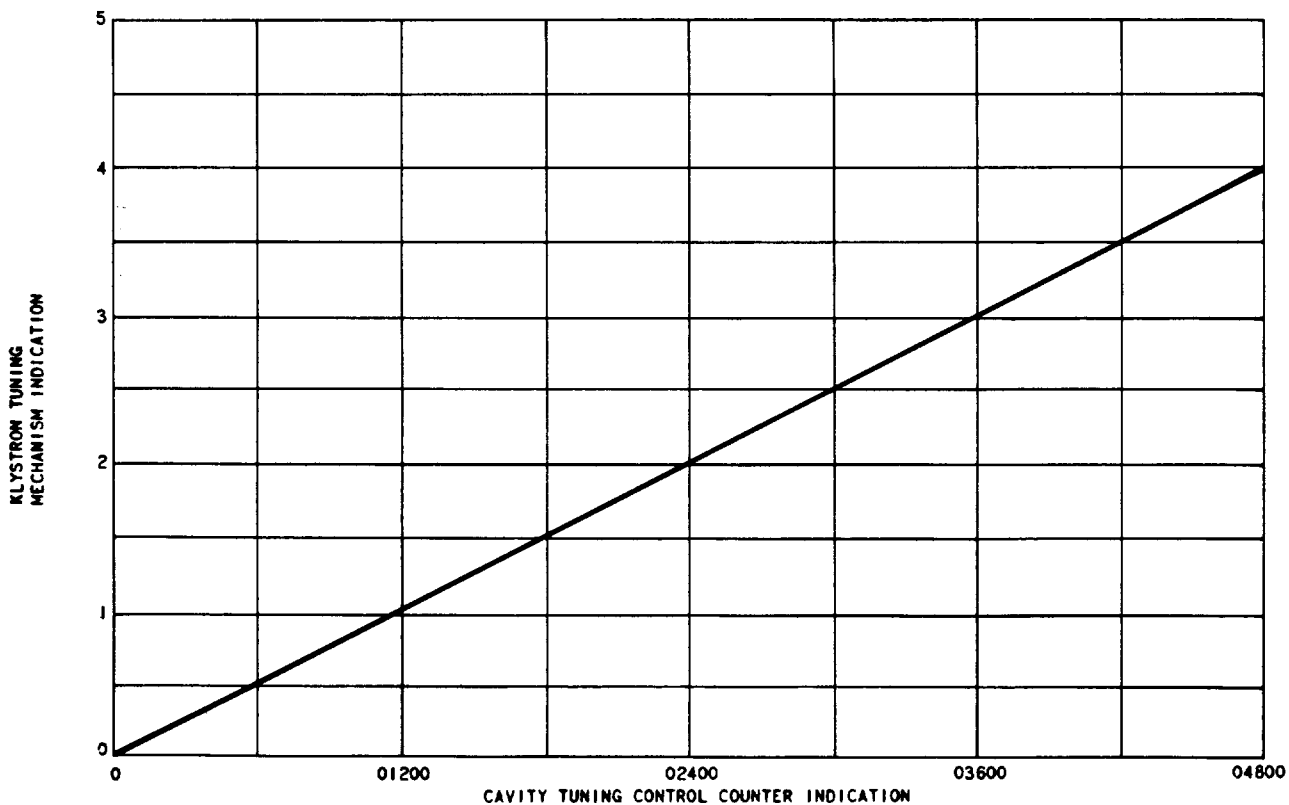
B - RELATION OF KLYSTRON TUNING CONTROL AND AMPLIFIER TUNING CONTROL ADJUSTMENTS
