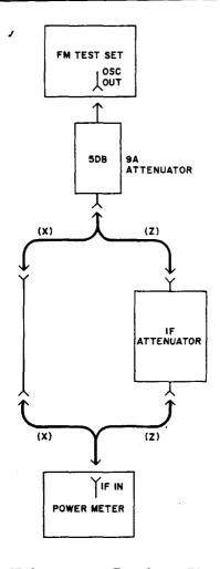
Fig. 1—IF Attenuator—Test Setup Diagram
