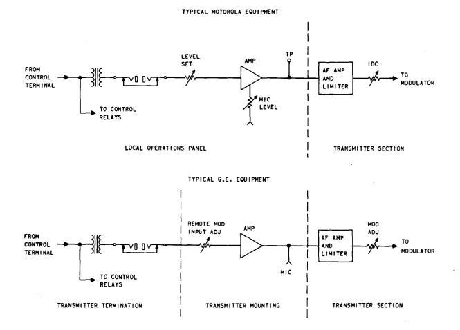
Fig. 2—Typical Transmitter Input Arrangements
