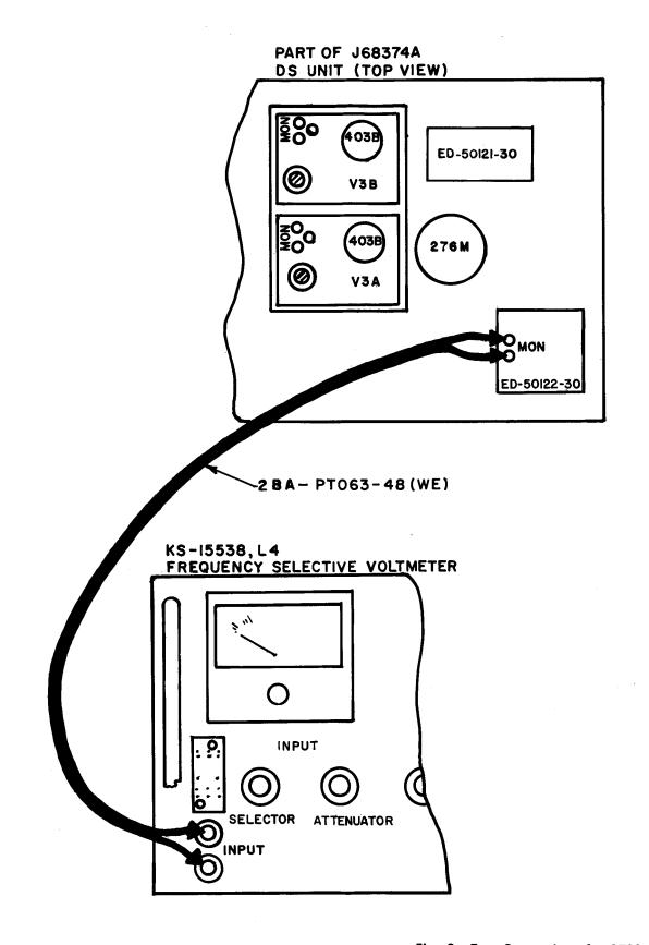
Fig. 3 – Test Connections for 3700-Cycle Pilot Tone Measurements
