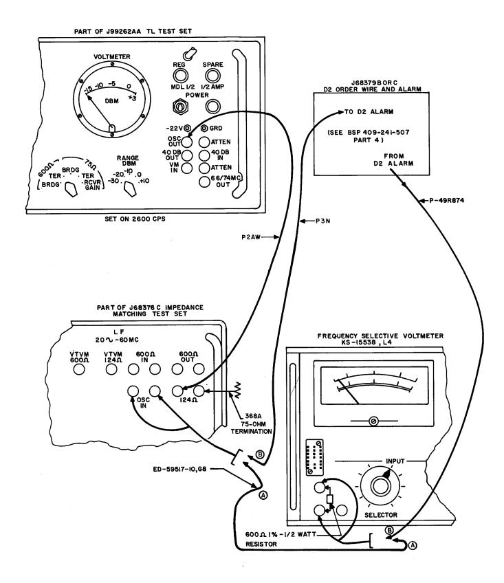
Fig. 6 – Test Connections for Setting 2600 CPS
