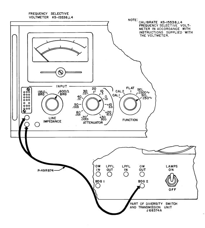
Fig. 1 — Test Connection for Signaling Tone Measurements
