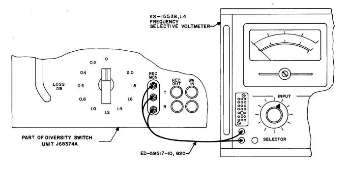
Fig. 4 — Test Connection for Measurement 3700 CPS
