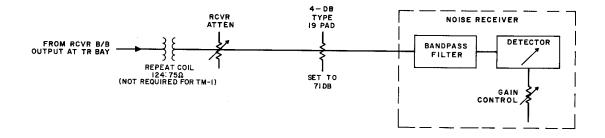
Fig. 1—TJ/TM-1 Noise Loading—Test Connections
