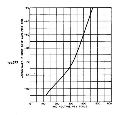
Fig. 1—Typical TL-1 Receiver—AGC Characteristics—Graph
