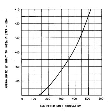
Fig. 3—J99351E Unit—Receiver AGC Characteristics—Graph
