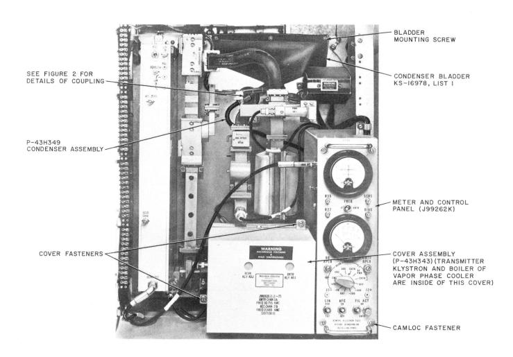
Fig. 1 — Transmitter-Receiver Panel
