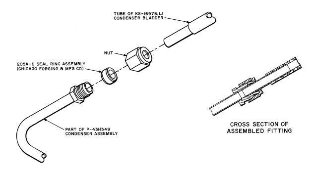
Fig. 3 — Coupling Between Condenser Bladder and Condenser Assembly
