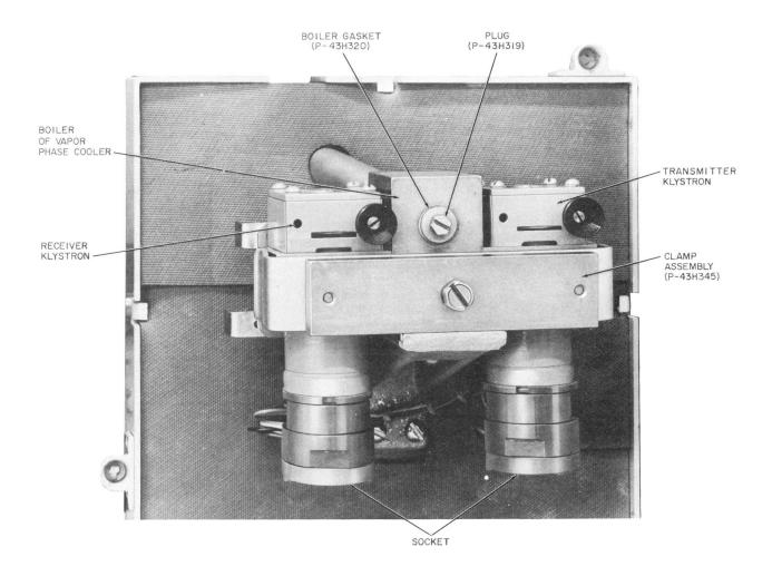
Fig. 2 — Transmitter and Receiver Klystrons and Boiler of Vapor Phase Cooler
