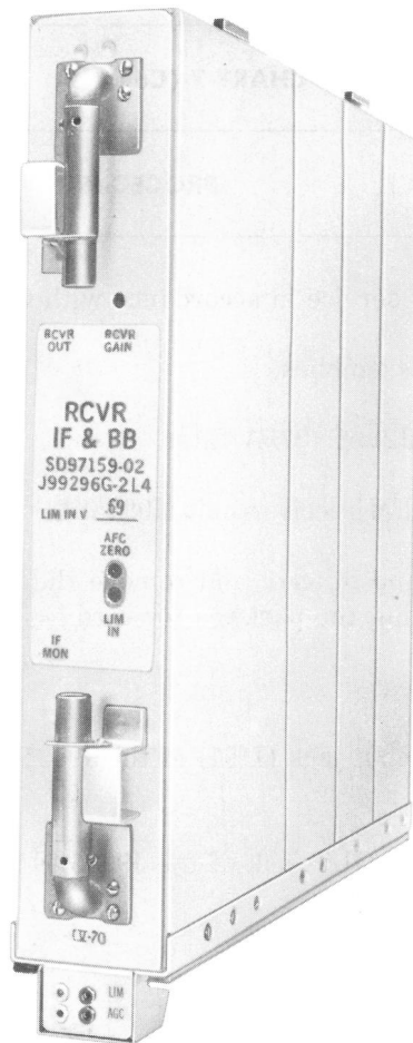
Fig. 9—J99296G Receiver IF and Baseband Unit
