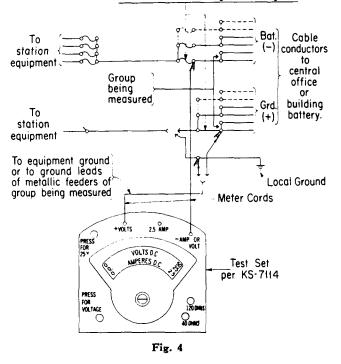
3.26 Divide the difference between the voltage readings by the current reading. Confirming the example in 3.24, the voltage reading taken while both the 120 OHMS and 40 OHMS keys are depressed would be 13.5 volts. The calculation is the same as for a single position PBX: Example:
