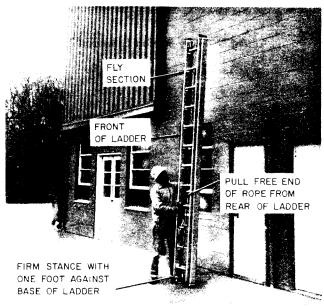
Fig. 19—Preparing to Extend Fly Section
