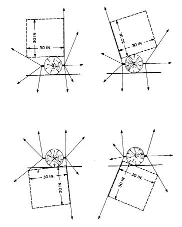
Fig. 4—Climbing Space When Drops are Attached Directly to Pole
