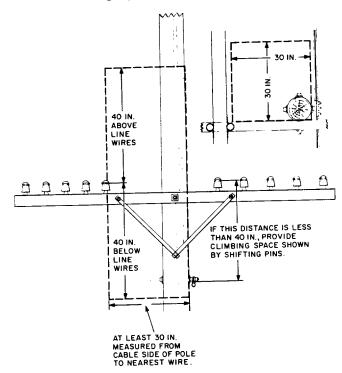
Fig. 6—Respacing Pins for Climbing Space
