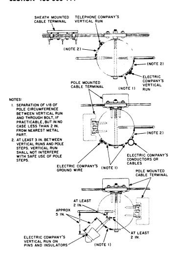
Fig. 1—Typical Vertical Run Clearances
