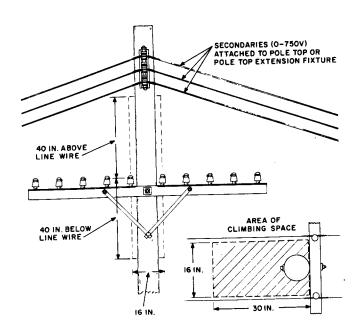
Fig. 3—Secondary Feeder Crossing Over Telephone Lines
