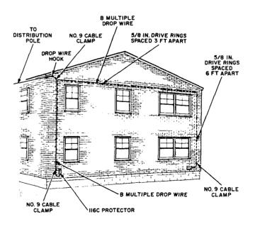
Fig. 1—Complete Wire Run on Building
