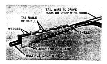
Fig. 2-D Drop Wire Clamp Assembled on Wire
