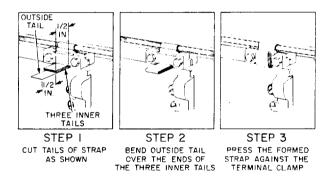
Fig. 5—Terminating Cable Supports
