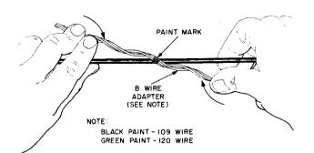
Fig. 3—Installation of B Wire Adapter
