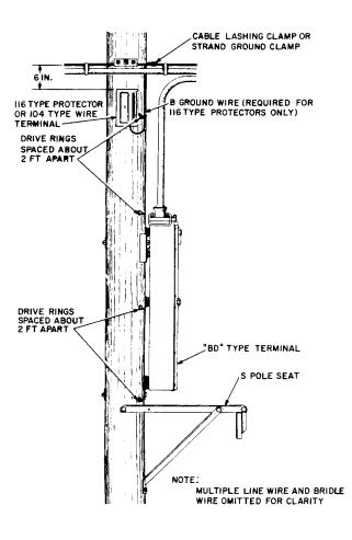
Fig. 11—Pole With Pole-Mounted Cross-Connecting Terminal (multiple line wire and bridle wire omitted for clarity)
