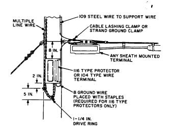
Fig. 12—Deadend Pole With Strand-Mounted Cable Terminal
