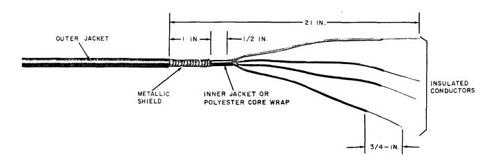
Fig. 15—Prepared Service Wire—E Cable Closure €
