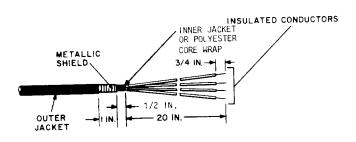
Fig. 19—▶Prepared Service Wire—LD Type Cable Closure •
