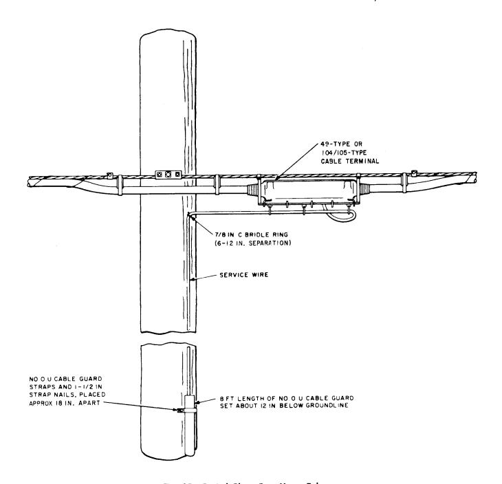
Fig. 25—Buried Plant Run Up a Pole
