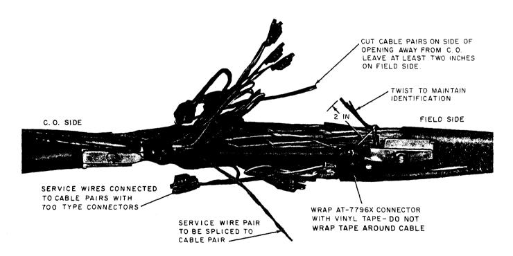
Fig. 5—♦Splicing Cable Pairs—13-Type Closure♦
