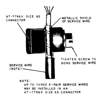
Fig. 4—♦Service Wire Installed in AT-7796X Connector♦
