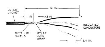
Fig. 7—Prepared Service Wire—RC4/72 Cable Closure €
