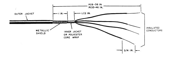
Fig. 9—₱Prepared Service Wire—PC6/48 or PC12/55 Cable Closure€
