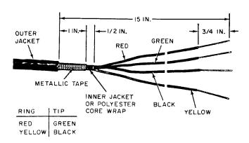
Fig. 21—Prepared Service Wire—UP200 Cable Closure
