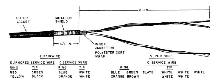
Fig. 3—Prepared Service Wire—13- or 14-Type Closure
