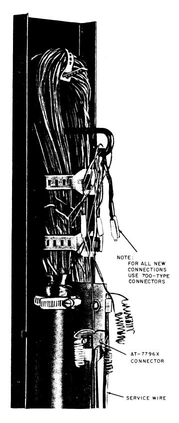
Fig. 22— Service Wire Installed—UP200 Cable Closure
