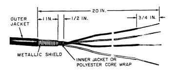
Fig. 14—Prepared Service Wire—D Cable Closure
