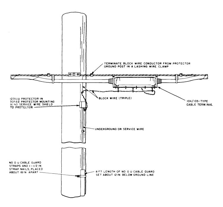
Fig. 28—Termination for Special Lightning Protection
