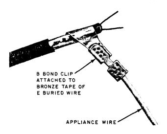
Fig. 27—₱Bonded Shield of E Buried Wire¶
