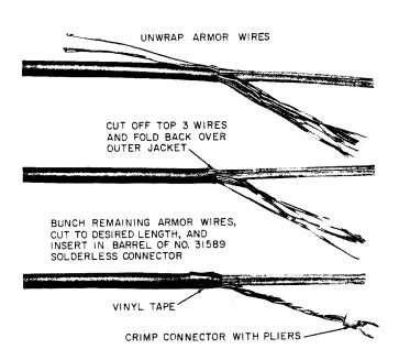
Fig. 35—Preparation of D Underground Wire (MD) for Protection or Cable Terminal Where Grounding is Required
