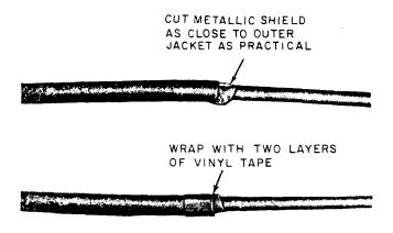
Fig. 26—▶Removal of Metallic Shield♥
