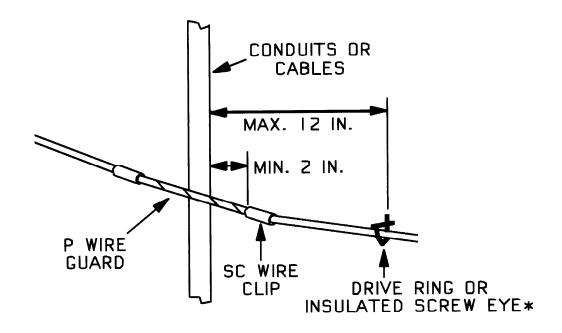
\* USE INSULATED ATTACHMENTS WHERE FUSED PROTECTION IS REQUIRED.
